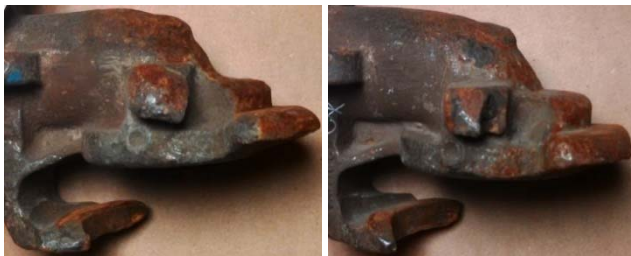
Figure 4. The Lip Bead Has Worn Off of Both Gladhands on this Pair of Service Separated End Hoses
