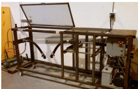
Figure 5. End Hose Separation Force Test Machine
