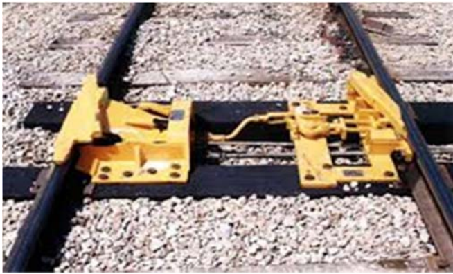
Figure 3. Typical Sliding Derail with Separate Crowder (Deployed)
