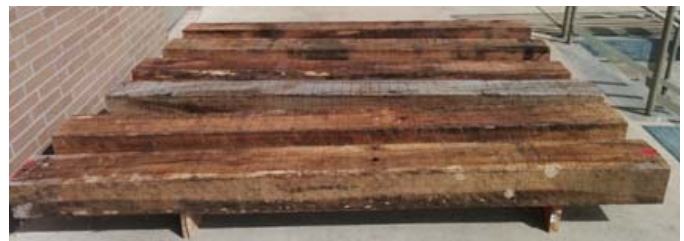
Figure 3. Untreated Oak Timber Ties
