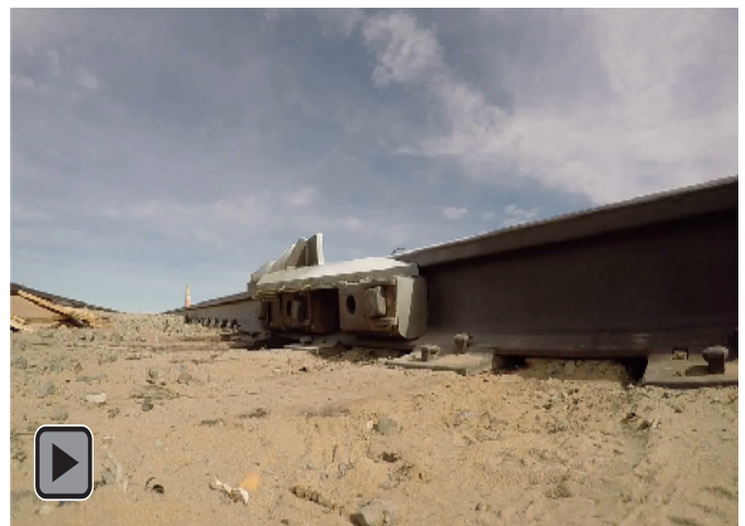
Figure 4. Video of Prototype Flange Bearing Derail at FAST and Railcar Passing over it at 4 mph
