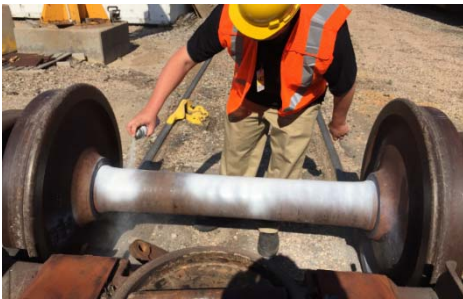
Figure 3. Application of the Speckle Pattern
