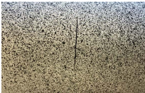
Figure 4. Notch in the Speckled Axle, Near Center
