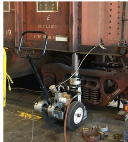
Figure 6. Hydraulic Jacks with Load Cells
