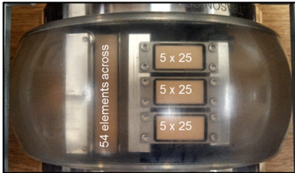
Figure 2. Phased Array Probes Configured Inside the RSU
