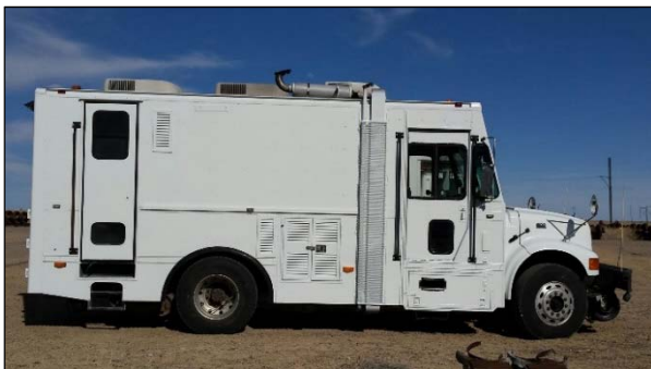
Figure 3. TTCI Hy-Rail inspection Vehicle
