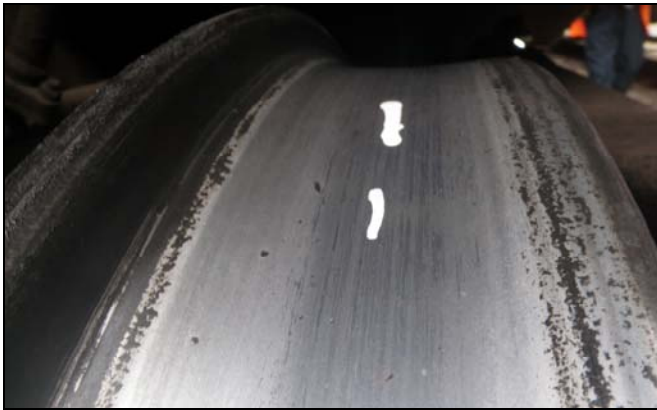
Figure 7. Tread surface showing minor pitting after 421,000 miles
