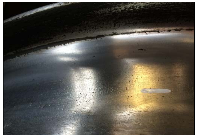
Figure 6. Surface cracks caused by scuffing
