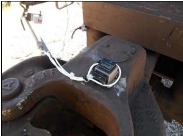
Figure 3. Triaxial Acceleration Instrumentation Mounted on Stationary Coupler
