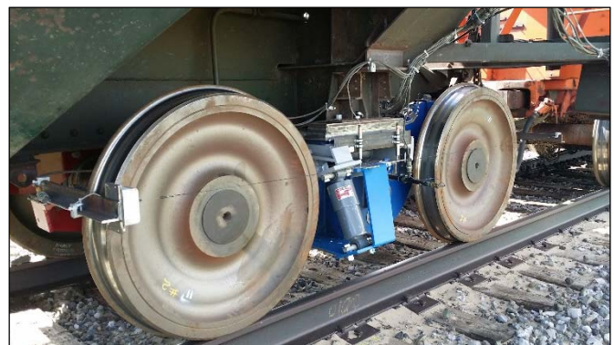
Figure 2. String Potentiometer Used to Measure the Angle between the Wheelsets
