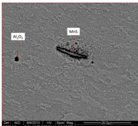
Figure 5. \text{Al}_2\text{O}_3 and MnS using SEM in HAZ of HAW
