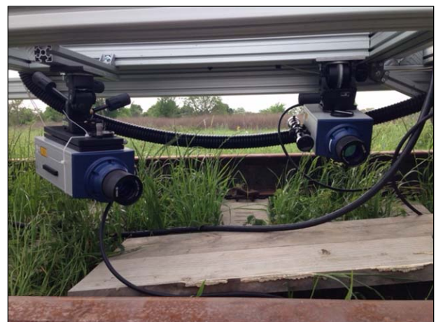
Figure 3. Laser vibrometers attached to the prototype cart
