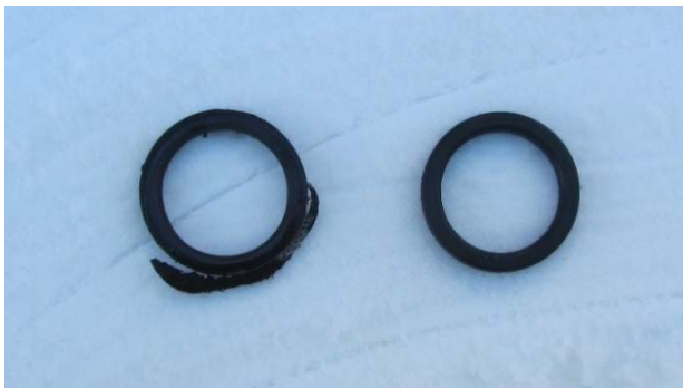
Figure 4. Damaged Gasket and New Gasket
