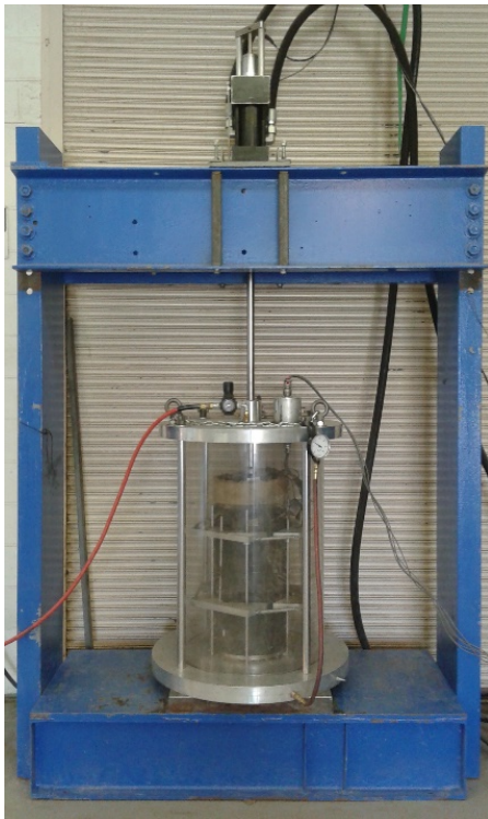
Figure 1. UIUC Triaxial Ballast Tester
