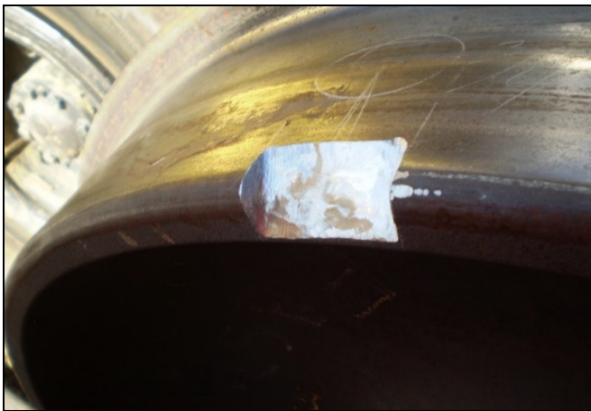
Figure 7. Rim notch on the test wheel (0.75-inch deep by 2-inch wide)
