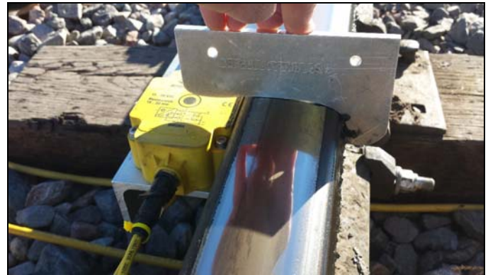
Figure 2. Magnetic wheel sensor and wheel segment
