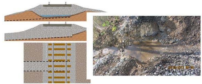
Figure 5. Ballast Drain Conceptual View and Installation
