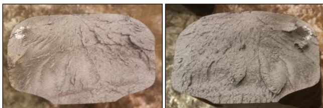
Figure 5. Weld Removed after Hand Scanning found a 9-percent CSHA NDT Indication within Weld
