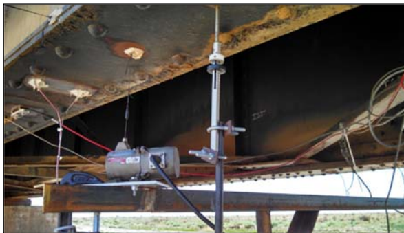
Figure 3. Fish Scale Vertical Deflection Indicator (right) and String Potentiometer (left) for Deflection Monitoring
