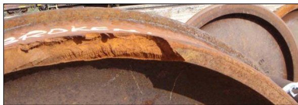
Figure 1. Wheel with a Broken Rim
