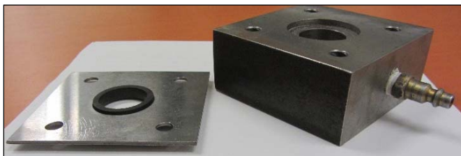
Figure 1. Test Jig with Gasket Disassembled
