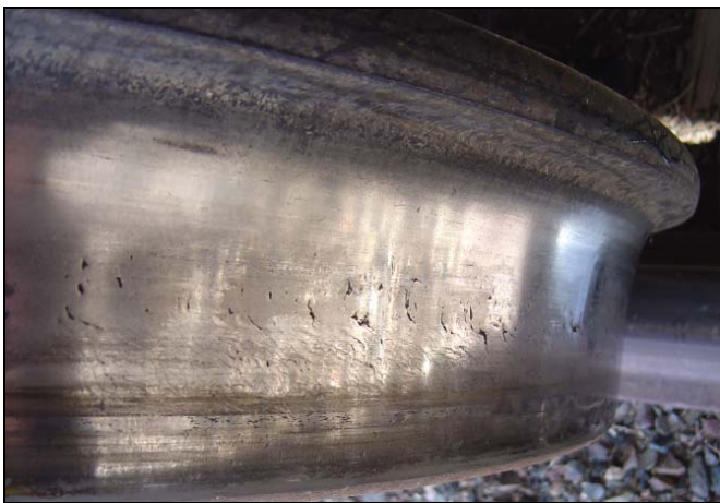
Figure 2. Scuffing-Related Tread Damage on a Test Wheel
