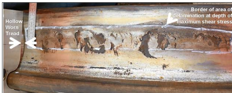
Figure 4. Delamination and Shelling
