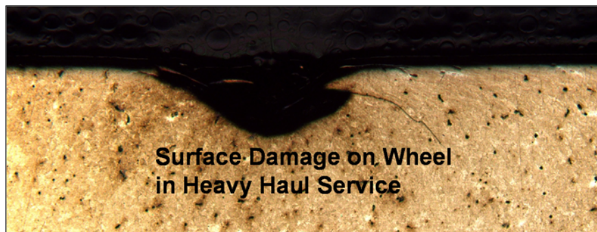
Figure 7. Material Flow and Crack Formation Associated with Scuffing
