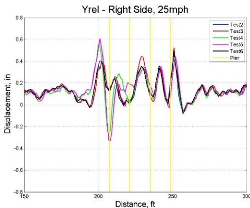
Figure 6. Yrel Measurements on Right Side for Different Bridge Conditions
