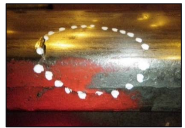
Figure 5. IS high rail shelling leading to transverse defect development in Type 1 and TZ rail. ERMS-SS rail type did not indicate a developing transverse defect underneath the shell.
