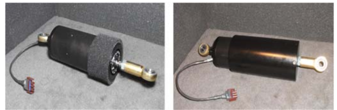
Figure 2. Fully Assembled Prototype Energy Harvesters used for On-Track Testing at TTC; (left) without Dust Cover, (right) with Dust Cover
