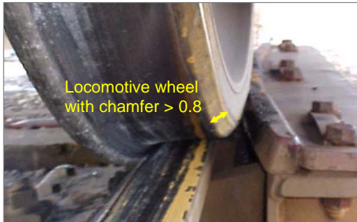
Figure 1. Locomotive Wheel Climbing a Field Side SPP
