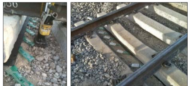
Figure 2. One of Five Test Zones with Three Test Ties in each Zone showing Excavated Crib Areas and the Installation and Location of Pressure Sensors
