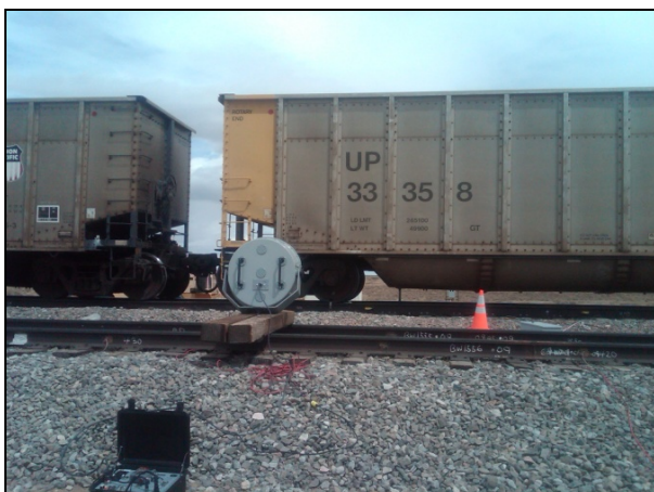
Figure 3. Air Coupled Acoustic Device in Position for Testing
