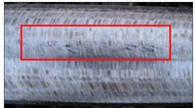
Figure 6. Low Rail at Wabun, Virginia, after Five Grinding Passes
