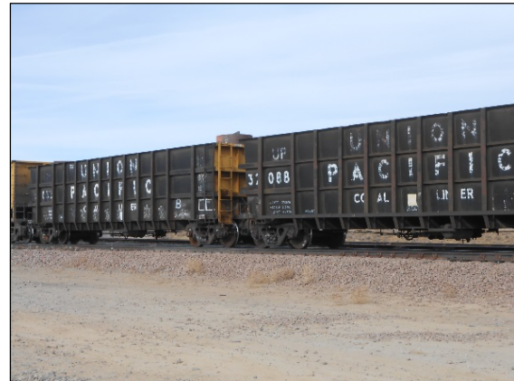
Figure 2. Steel Gondola Cars Overloaded to 400-kip GRL
