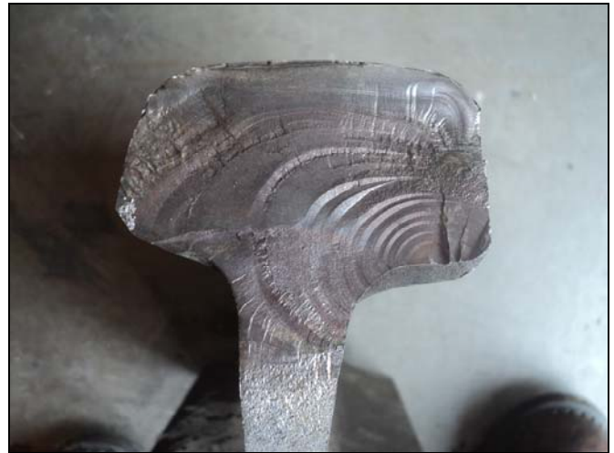
Figure 7. Fatigue Fracture Initiated at Stress Concentrator at bottom of Railhead
