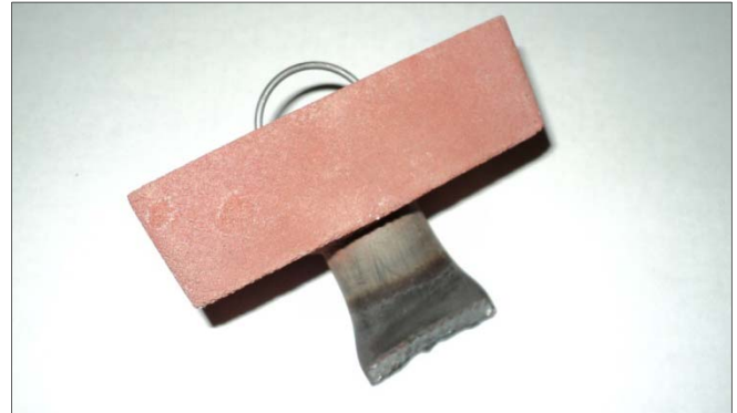
Figure 2. Alloy Container Incorporated into Bottom of Diverter Plug (The container melts when head riser fills, dispersing the alloying elements into the head of the weld)
