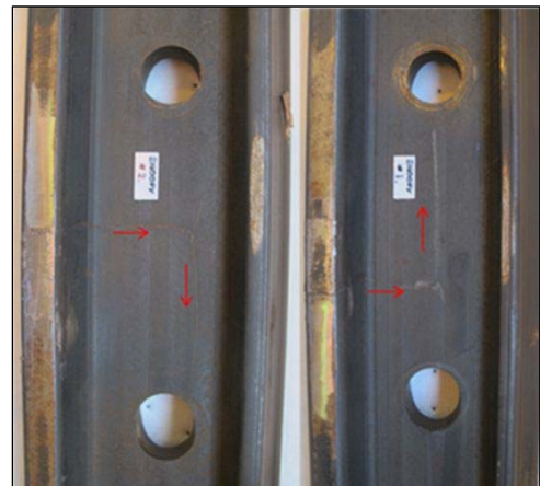
Figure 3. Cracked Joint Bars
