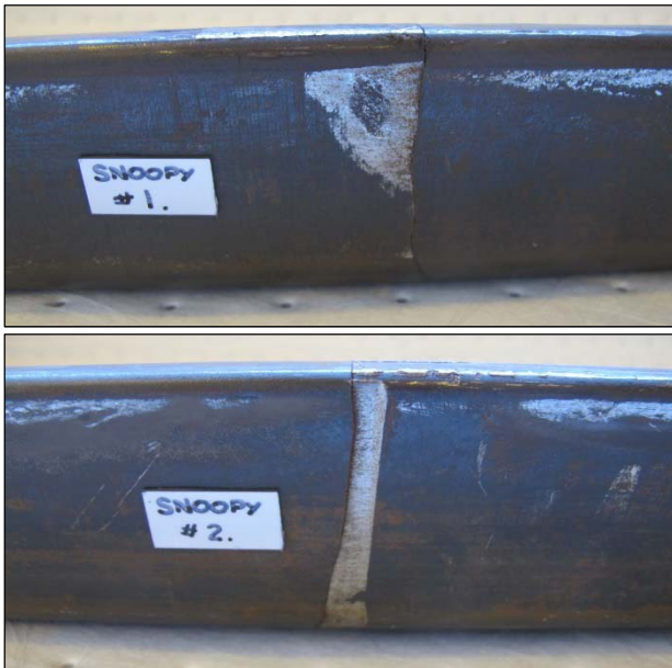
Figure 4. Indentation at Joint Bar/Rail Contact
