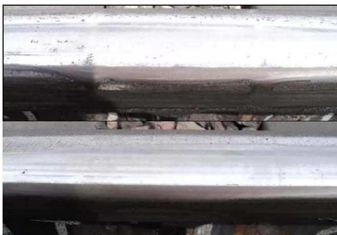
Figure 7. Railhead Running Surface. Top – Untreated Thermite Weld at 70 MGT Bottom – Treated Thermite Weld at 70 MGT
