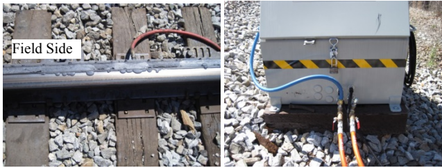
Figure 4. (a)TORFM Applicator, (b) Rerouted Hose for One Rail Application Test
