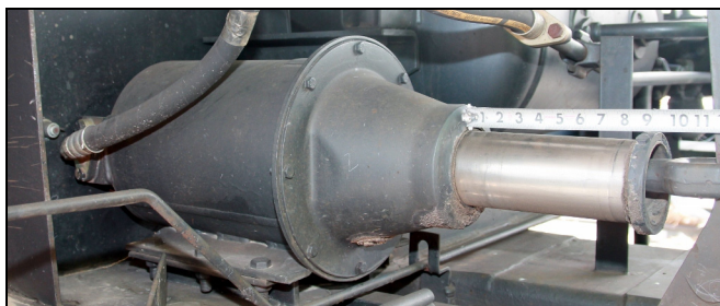
Figure 1. Piston Travel Measurement
