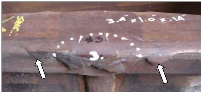
Figure 1. Thermite Weld Showing Batter of HAZ (indicated by arrows) and Shelling at Gage Corner of Weld
