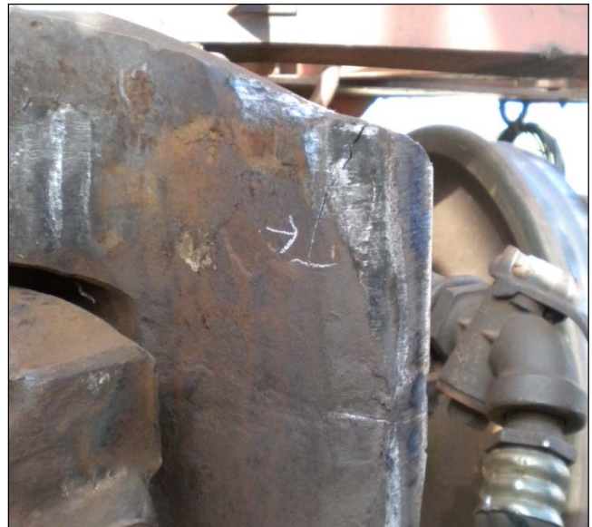
Figure 1: Cracked Guard Arm of Coupler
