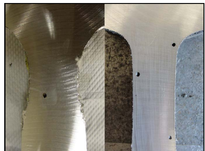
Figure 5. Gas Holes in Railtech Welds R4 (left) and R12 (right)
