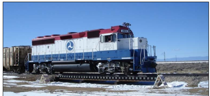
Figure 1. BDTF – Adjustable Three-Span Trestle for Evaluation of Onboard Bridge Detection Systems
