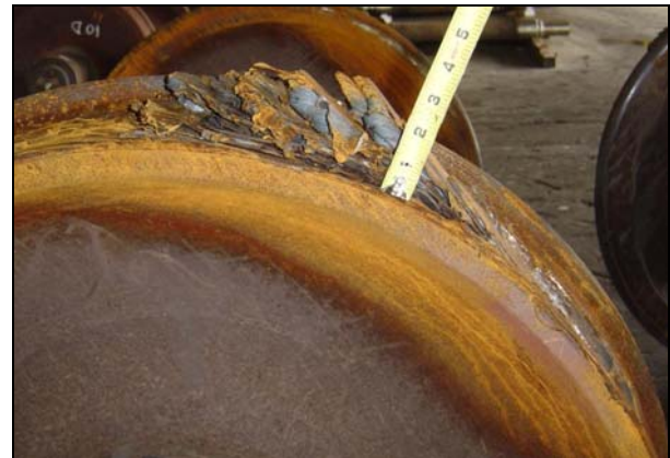
Figure 1. Wheelset with TBU Extending 3 Inches Radially from the Tread Surface
