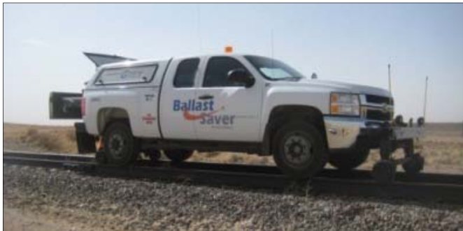
Figure 1. GREX's BallastSaver Hi-rail Vehicle Platform
