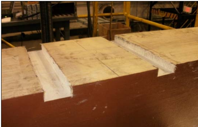
Figure 7. FFU Tie Milled to Clear Rivet Heads on Top Flange
