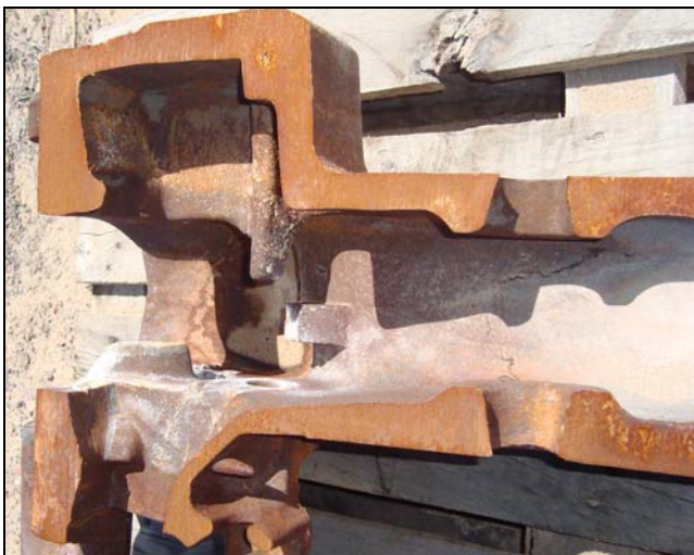
Figure 1. Example of Coupler Cross-Sectioning
