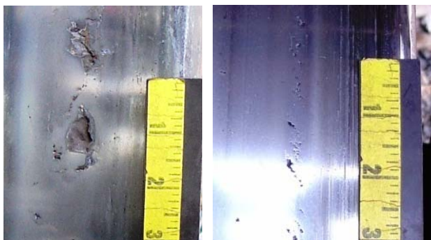
Figure 1. Medium Shells (left) and Small Shells (right) with an Inch Ruler for Size Reference
