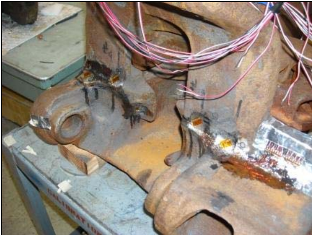
Figure 3. Strain Gages Installed on Coupler
