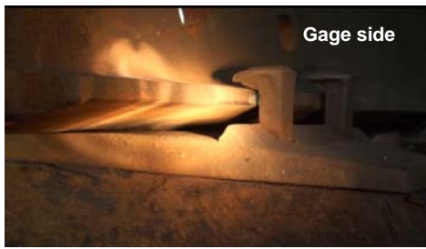
Figure 2. Frame from a Video Showing Low Rail Rotation under Loaded Coal Train
