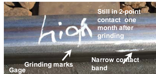
Figure 5. High Rail Showing Strong Two-Point Contact
