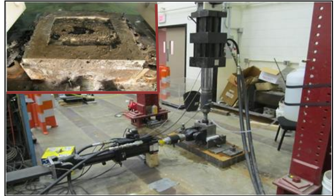
Figure 1. Rail Seat Abrasion Test
