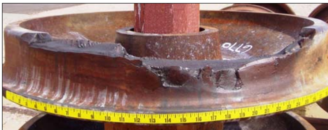
Figure 2. Wheel with VSR Failure
