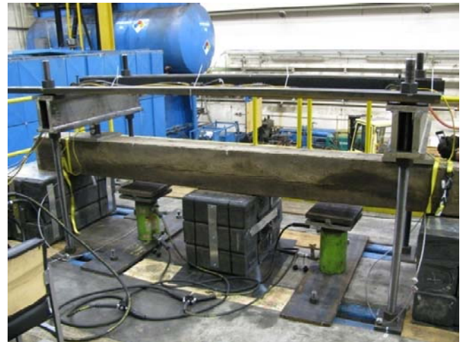
Figure 2. TTCI Demonstration Open Deck Bridge Tie Test Fixture
