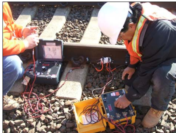
Figure 1. Resistance Measurement at the Amtrak Test Site
